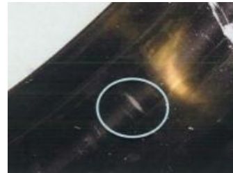
Mild wear caused by parked-state
