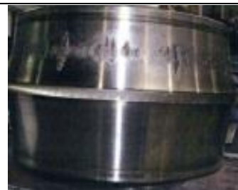
Inner Ring Raceway loads are excessive
