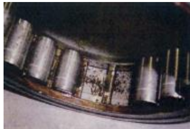
Spalling & flaking caused by inadequate lubrication
