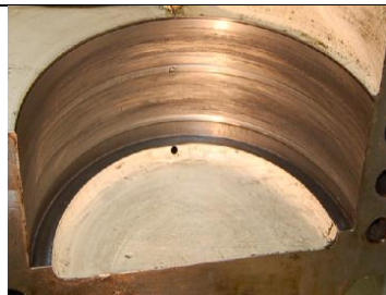
housing Scoring caused by heavy loaded bearings
