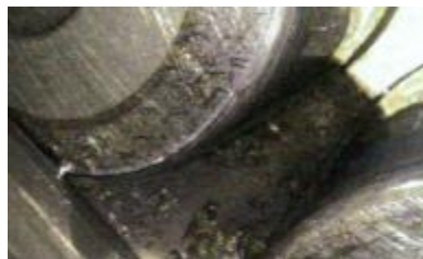
Smearing, cylindrical rollers caused by ineffective lubrication
